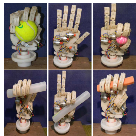
Fig. 2. TU Bionic Hand performing six Grasp Types involved during 70% of dla
