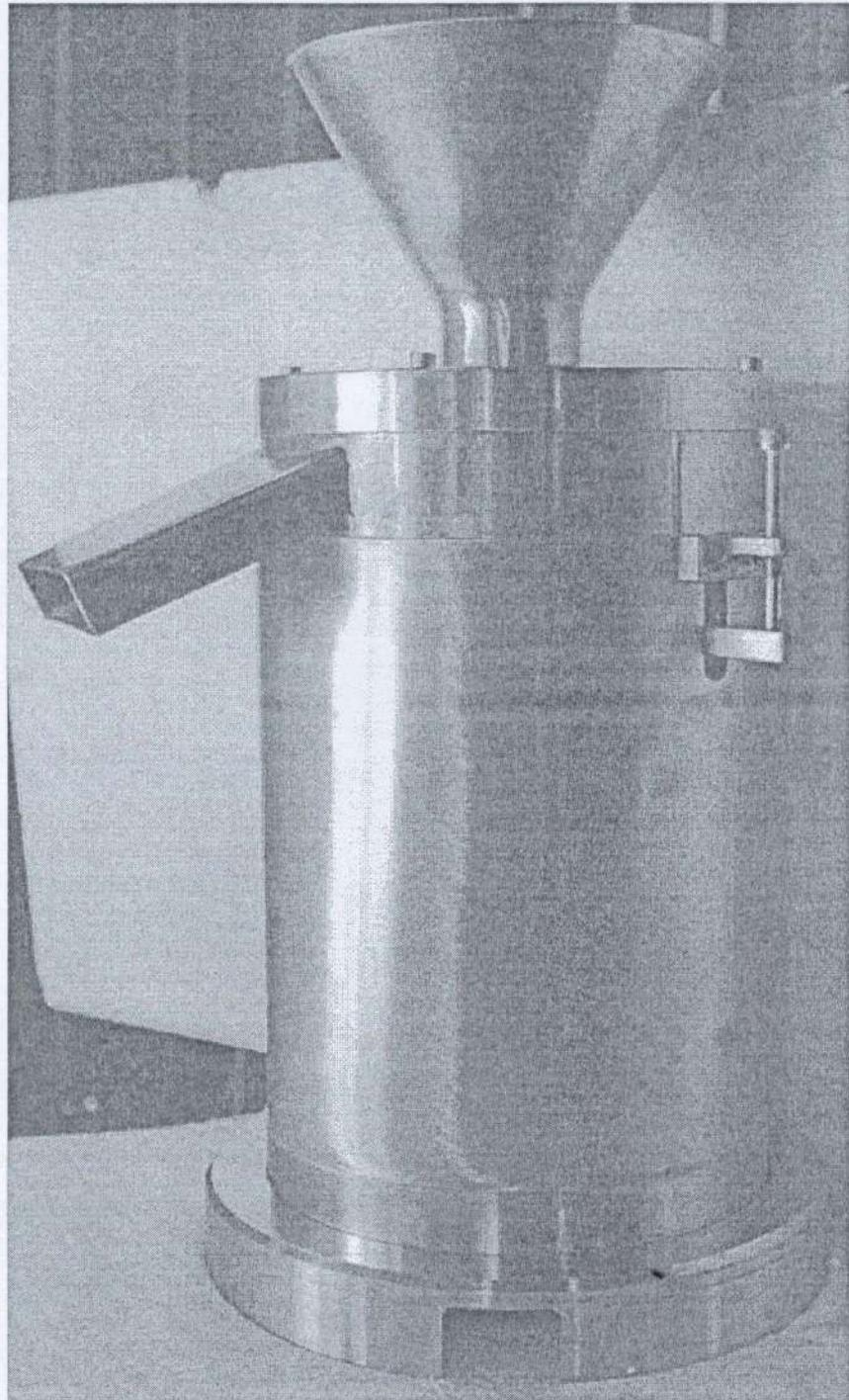
Fig. 4 : Table top continuous wet cum dry grinder.
