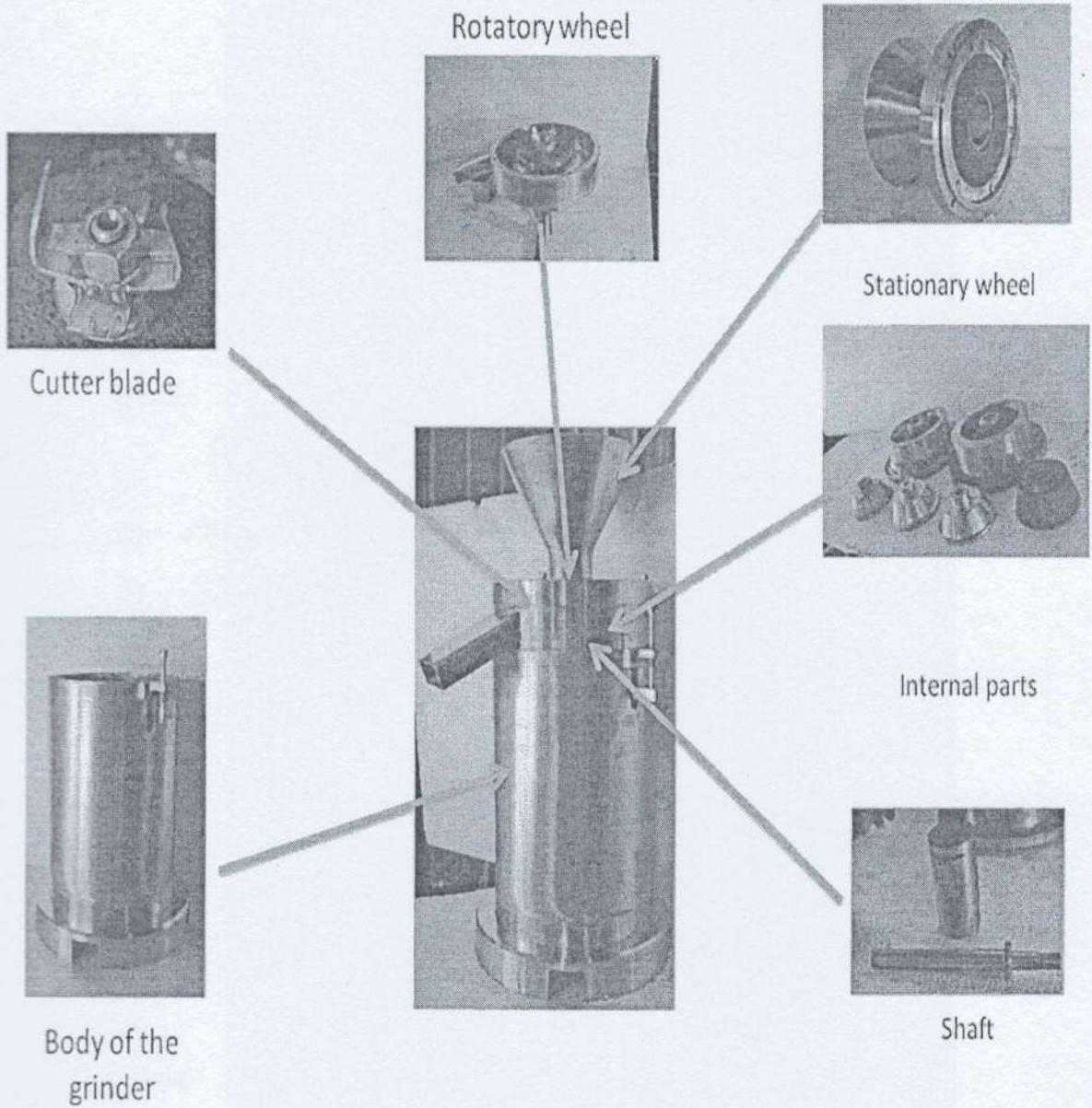
Fig. 5 : Various parts of continuous wet cum dry grinder.
