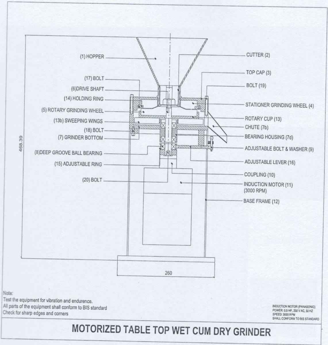
Fig. 3 : Engineering drawing of truncated conical continuous wet cum dry grinder
