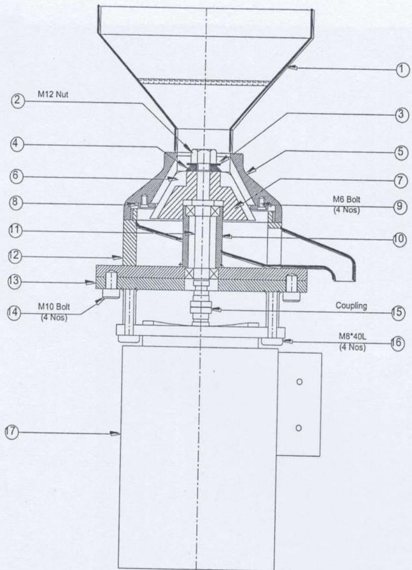
Fig. 6 : Engineering drawing of Modified-Improved continuous wet cum dry grinder.
