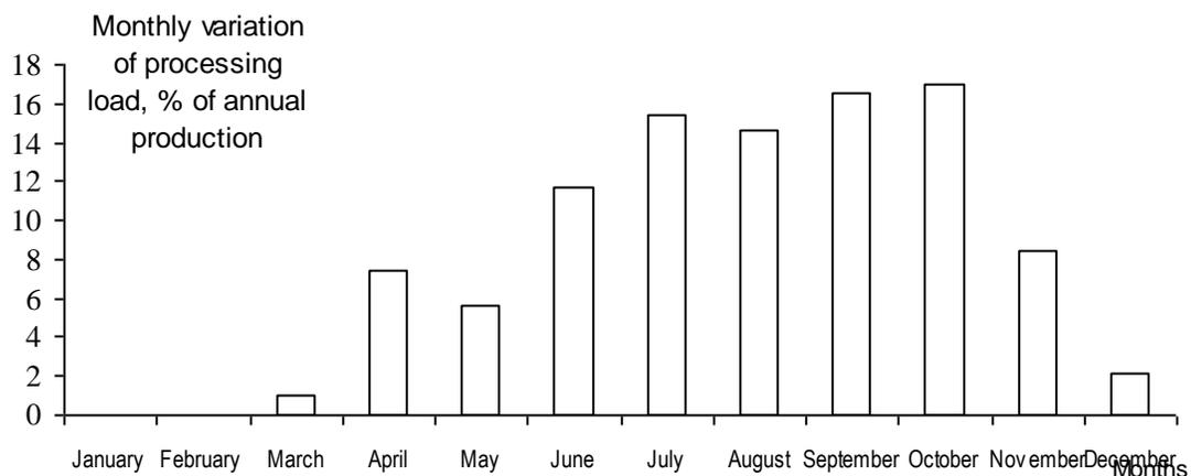
Fig.1 Monthly variation of processing load in a tea processing units with two million kg of annual production
