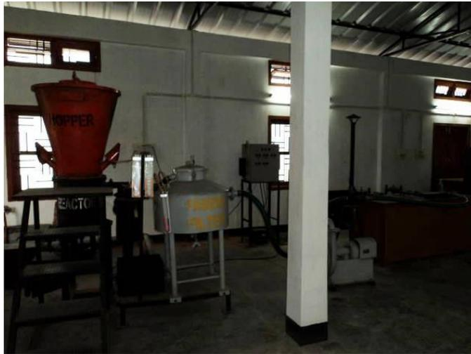
Fig. 5 Commercial biomass gasification unit for generation of producer gas
