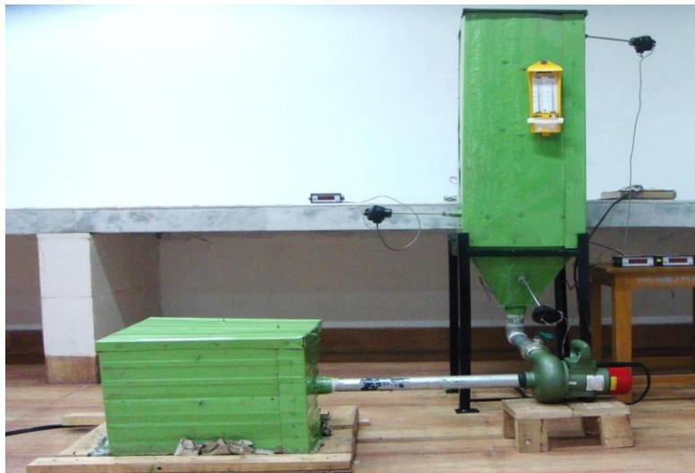
Fig. 7 laboratory setup of two stage fluidized bed dryer.
