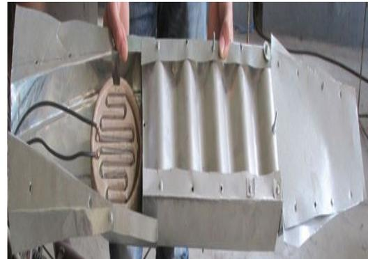
Fig. 3 Test section for sinusoidal geometry
