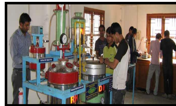
A transesterification experiment in progress at Biodiesel Plant
