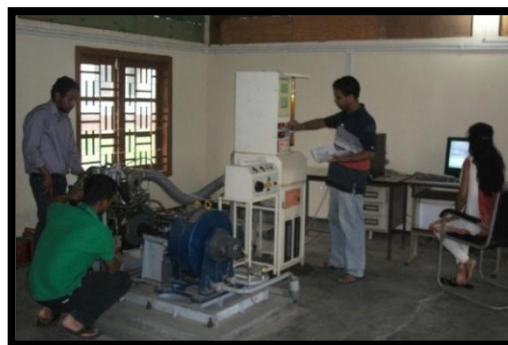
Performance testing of C.I. engine at Computerized Diesel Engine Test Rig
