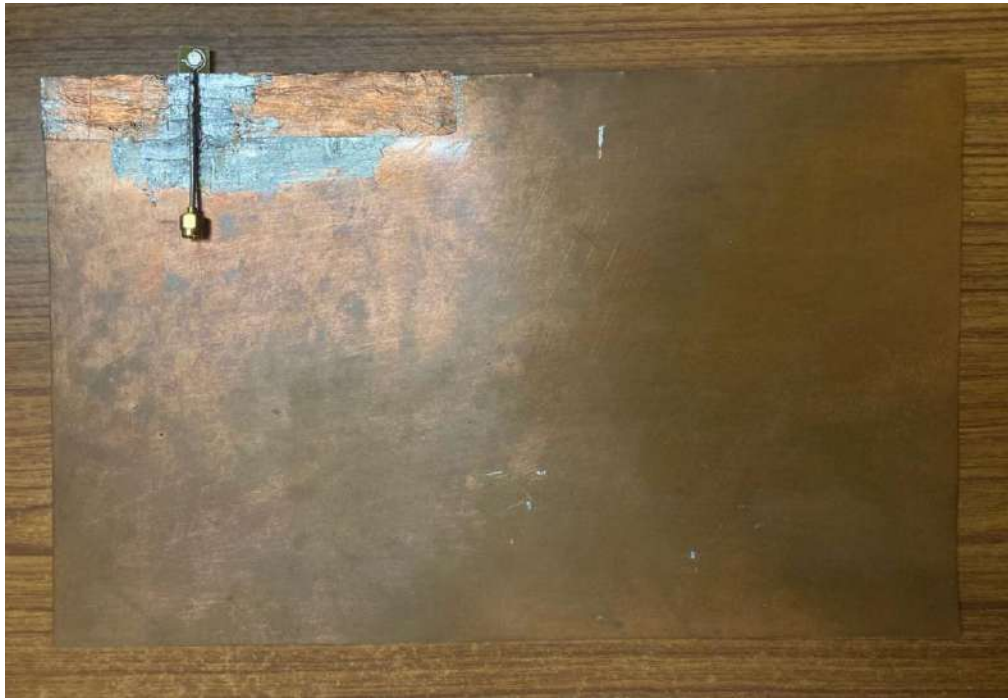
Compact laptop Antenna Prototype for WiFi 6E,7,8 Quadruple Band Applications
