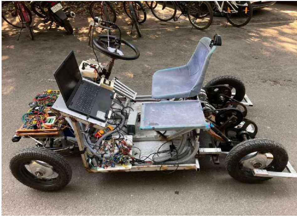
Battery Electric Vehicle (BEV) for Traction Control experiments integrated with a custom motor driver and sensors for performance monitoring
