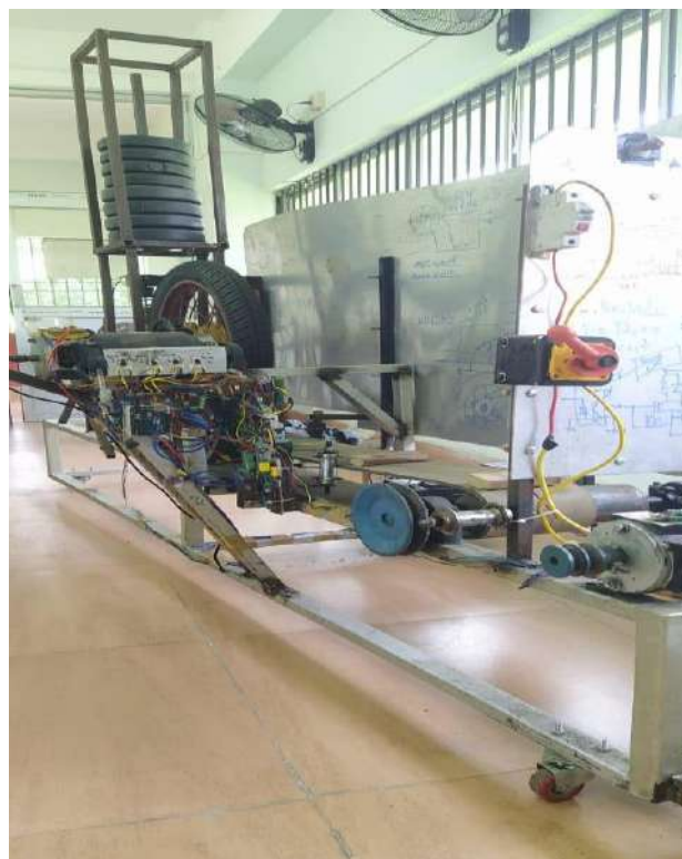
Quarter car model inspired suspension test bench for analysis of damper dynamics
