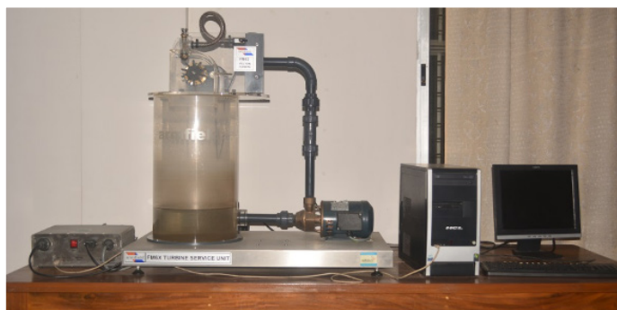
Pelton Turbine Apparatus
