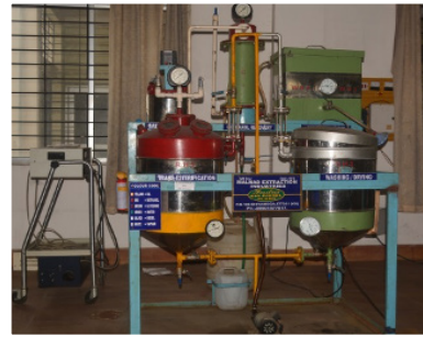
Biodiesel transesterification unit
